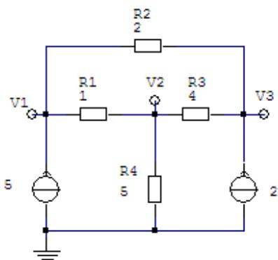
A nodal analysis can be performed by examining each node in a circuit. The goal is to find out what the voltages are in each node with respect to our reference node. We need to know the currents flowing in the circuit and the resistances between each nodes. This is just an application of the Ohm's Law.
