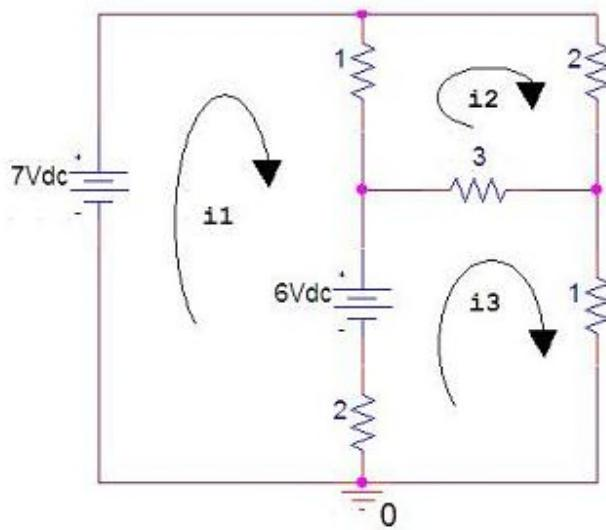
Given the relationship, voltage=Resistance multiplied by current, and the circuits shown above, find the values of the currents  $i_1$ ,  $i_2$ ,  $i_3$
