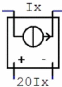
In particular, this source is creating a voltage of 20 times the current  $I_x$ , that goes through the top branch of the circuit, that is, through the 4-ohm resistor.
